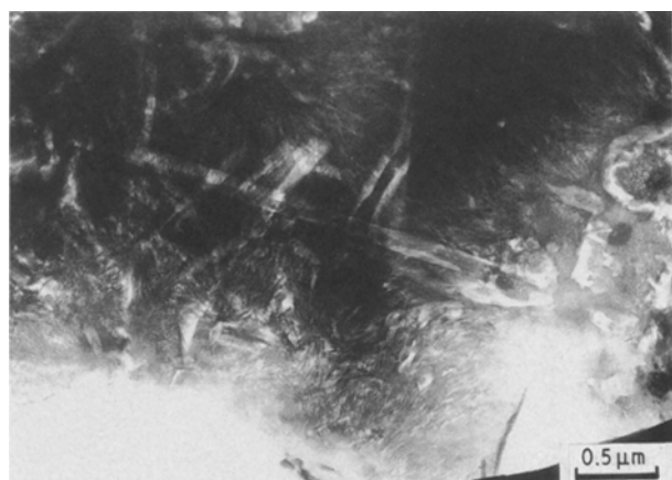
Figure 2 Transmission electron micrograph showing both fine-fibrillar and foil-like Op, C-S-H in a 75% slag blend (W/S = 0.4, 20 °C, 14 months).
