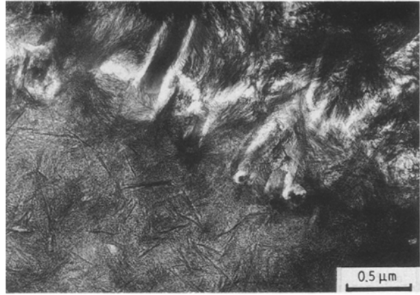
Figure 8 Transmission electron micrograph showing Mg, Al-rich precipitates randomly distributed within a slag inner product region (lower left-centre), fine fibrillar Op C-S-H (upper right-centre), an AFm plate (upper left-centre) and several AFt relics along the Ip/Op interface (50% slag blend, W/S = 0.4, 20 °C, 3 months).
