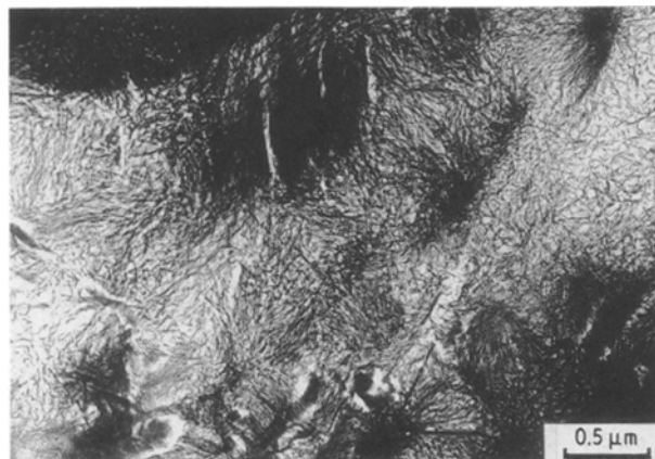
Figure 4 Transmission electron micrograph showing AFt relicts in the outer product region of a 10% slag blend (W/S = 0.4, 20 °C, 14 months).
